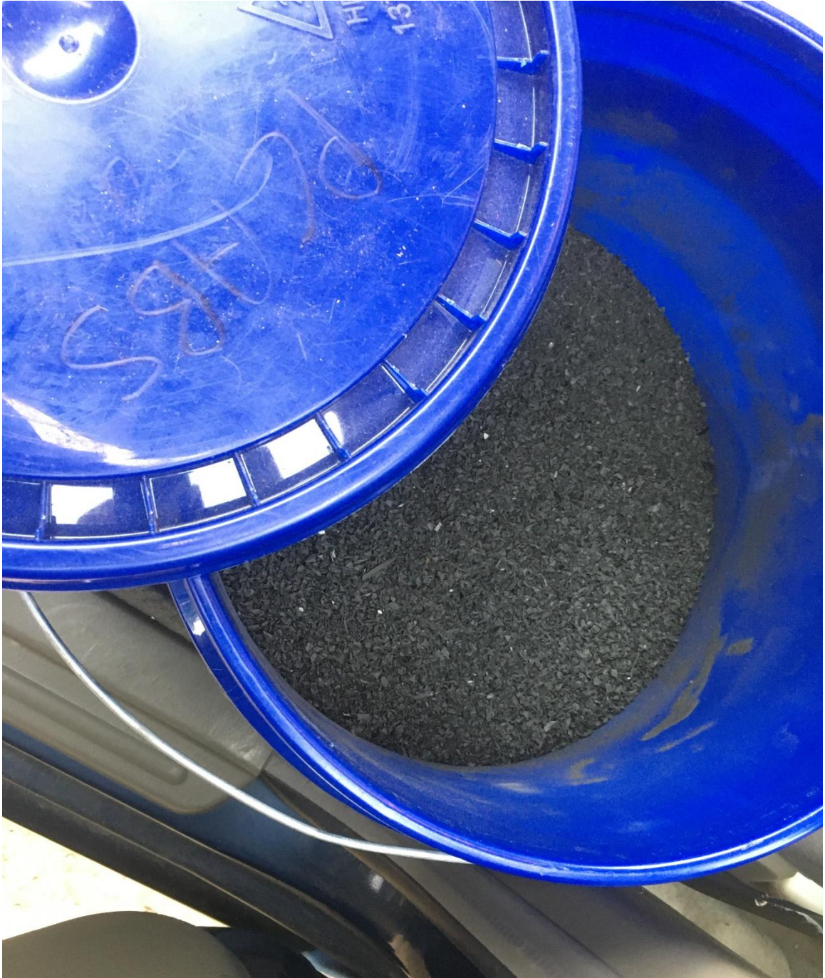
Figure 33. Raw regrinded feedstock material for the nylon, glass fiber, and glass bead composite obtained from the Murakami Corporation manufacturing plant in Campbellsville, KY.
