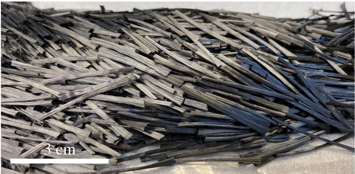
Figure 2. Sample of one category of sized carbon fibers from Oak Ridge National
