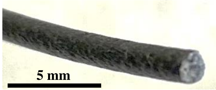
Figure 10. Enlarged photo of the surface of the sized carbon fiber composites.
