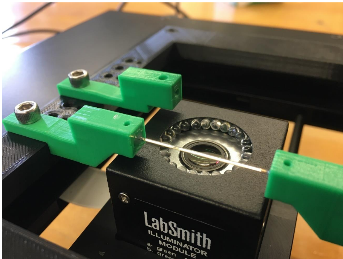
Figure 40. Leak-proof glass capillary mounts designed for a dielectrophoresis experiment in collaboration with NASA. Two-part epoxy was used to attach the glass capillaries to the printed products that were designed in SolidWorks, sliced in Ultimaker Cura, and printed on a Creality Ender 3 printer. Also pictured: black printed frame was designed in SolidWorks to mount the capillary adapters above the microscope via metric-sized screws from McMaster-Carr that were lined with Loctite.
