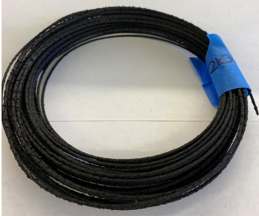
Figure 34. Filament obtained from the nylon-glass composite feedstock that was extruded at 210°C. Surface finish is too rough to be usable for printing due to the glass fibers and glass beads protruding through the surface and not mixing well enough with the polymer.
