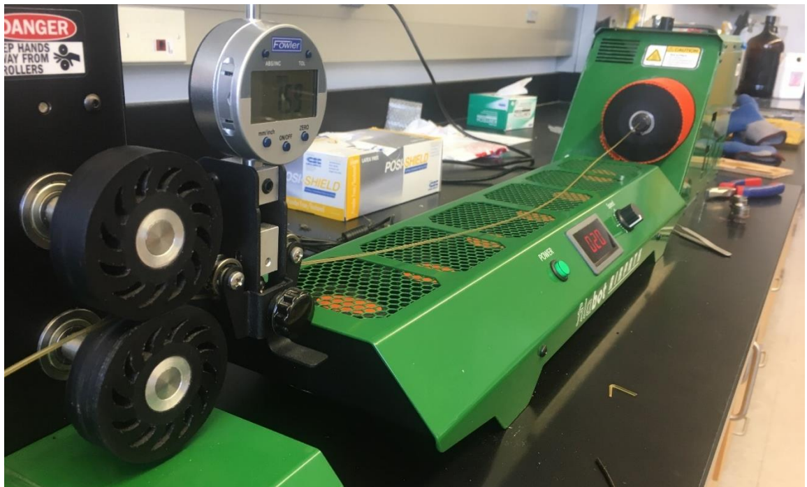
Figure 6. Filabot Extruder Setup that was used to create the composite filament with sized carbon fibers (different polymer pictured).
