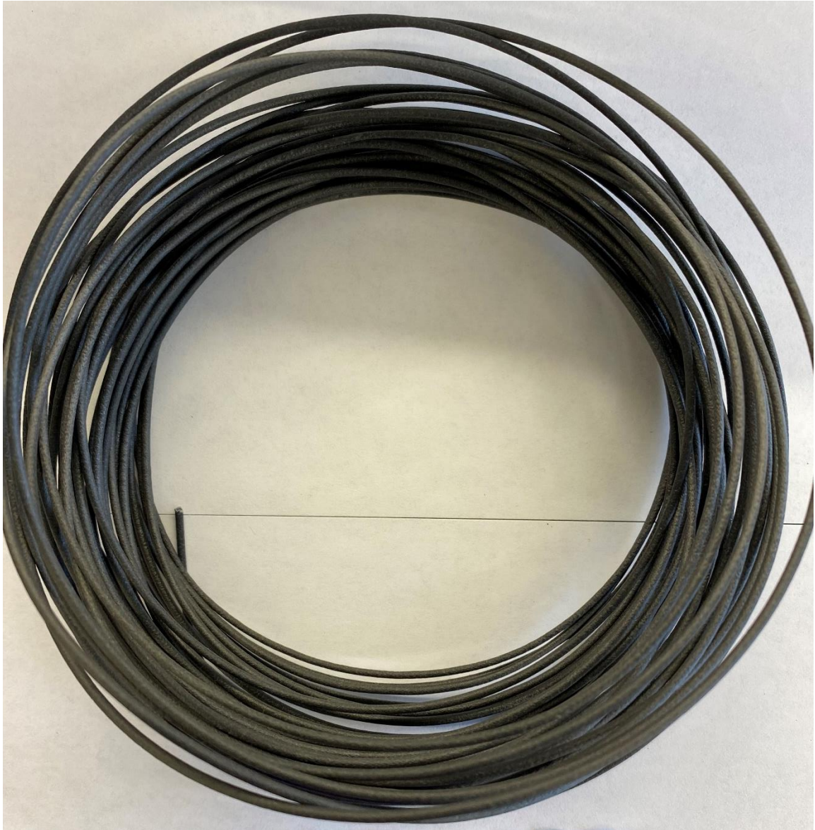
Figure 9. Filament produced with fibers coated with the Duroxyn ® SEF 968/25WA sizing agent.
