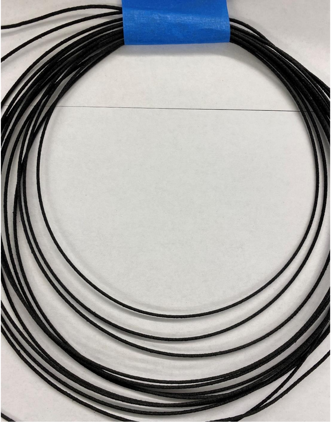
Figure 36. Filament obtained from the nylon-glass composite feedstock that was extruded at 230°C. Surface finish is smooth but is still abrasive enough to cause skin injuries due to some of the glass fibers on the surface. It is completely usable for printing.
