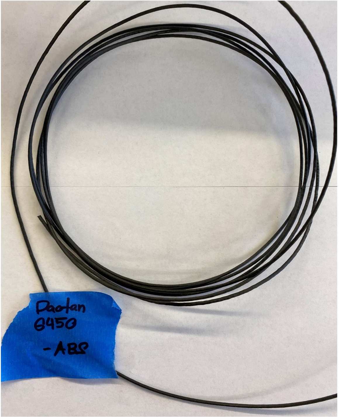
Figure 7. Filament produced with fibers coated with the Daotan ® TW 6450/30WA sizing agent.
