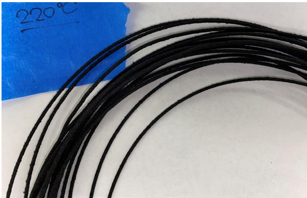
Figure 35. Filament obtained from the nylon-glass composite feedstock that was extruded at 220°C. Surface finish is rough enough to cause skin injuries when handled roughly due to the glass fibers on the surface, but it is usable for printing.
