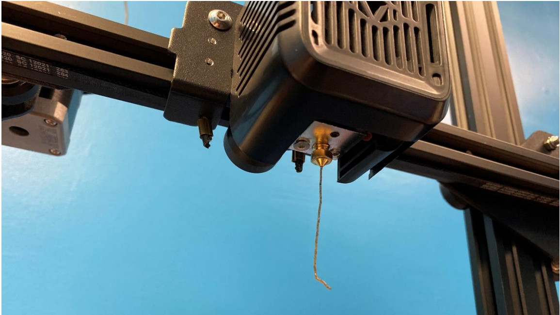
Figure 31. Soybean husk fiber with PLA composite successfully extruded from the nozzle of the additional printer that was purchased for use with natural fibers.
