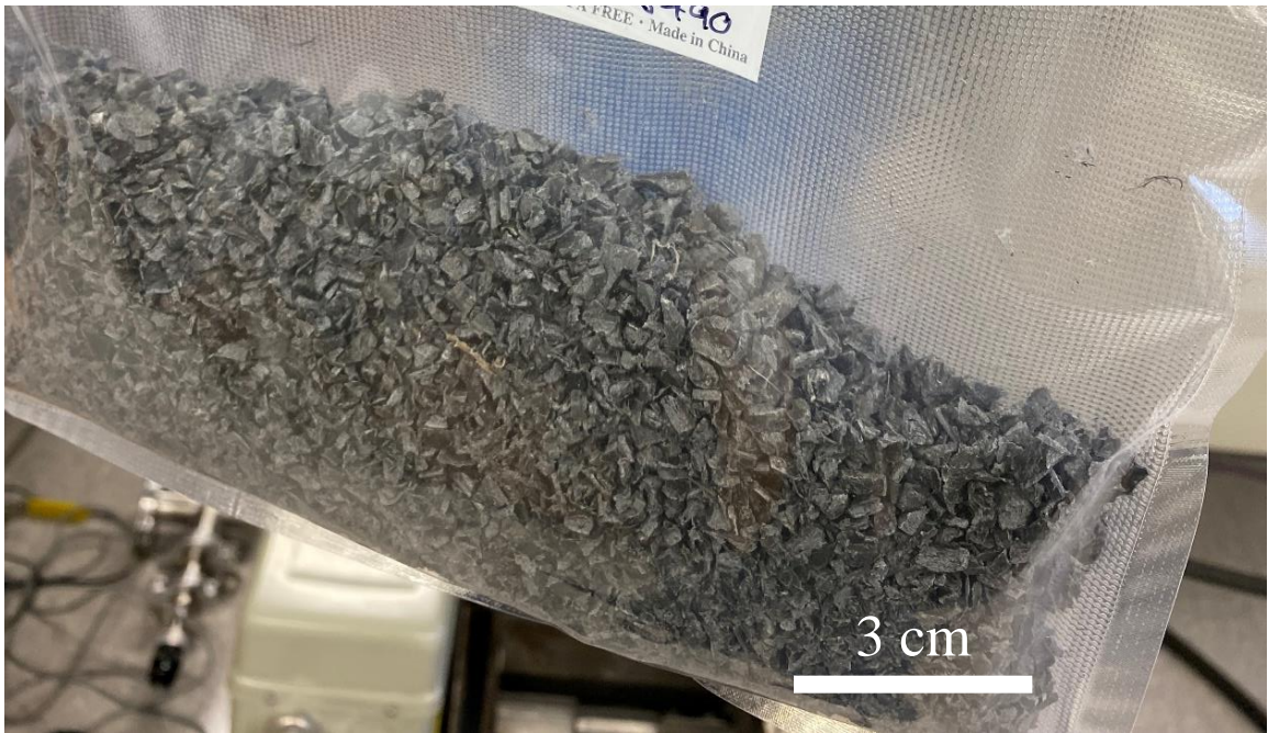
Figure 5. Pelletized material for the composite with fibers sized with Daotan TW 6490/35WA.
