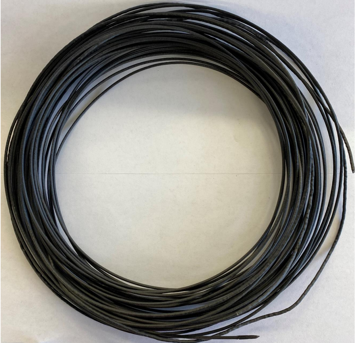
Figure 8. Filament produced with fibers coated with the Daotan ® TW 6490/35WA sizing agent.
