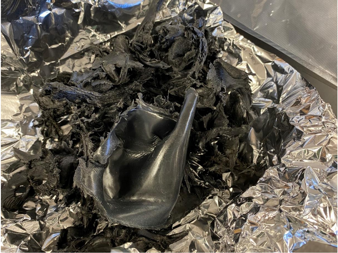
Figure 3. Sample of one of the resulting composites from the torque rheometer mixing, placed into a sheet of aluminum foil to safely cool for handling before further processing.
