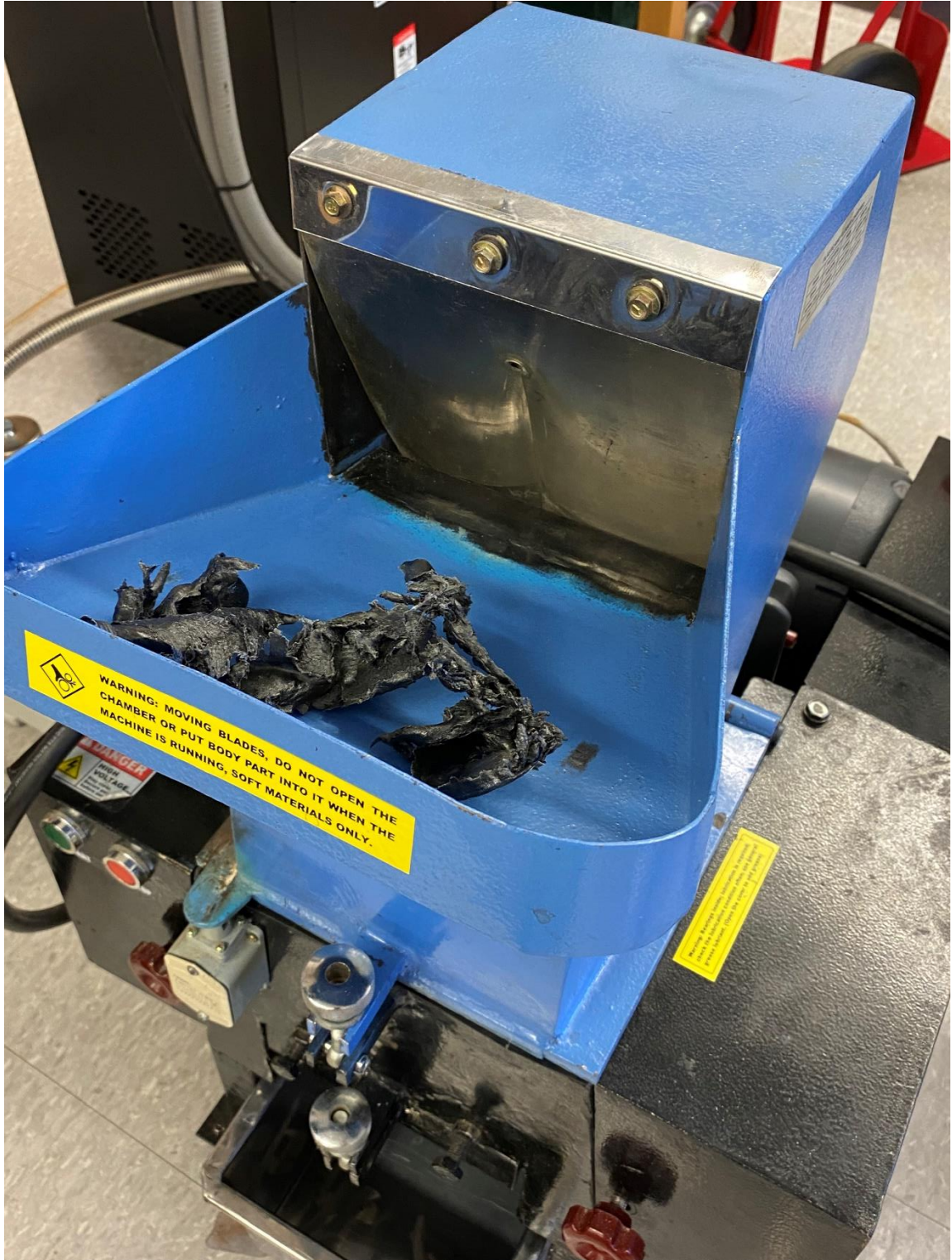
Figure 4. Insertion of a hardened composite sample into the industrial grinder.
