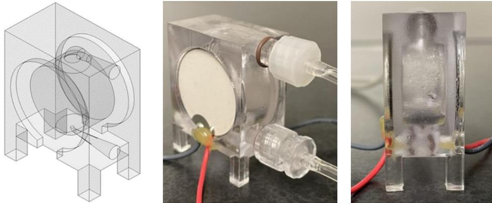
Figure 31: Rendering of acoustofluidic attenuation device as in SolidWorks (left) and two angles of 3D printed device with attached transducers and tubing (middle and right).
