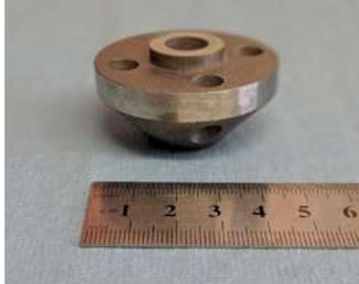
**Figure 6.1.** L-PBF fabricated water atomized 25Cr7Ni stainless steel based flange design to be used in underwater offshore oil rigs – the original design was modified to be printed without the use of supports while fabricating through L-PBF primarily to limit post-processing enabling on-site L-PBF fabrication on oil rigs
