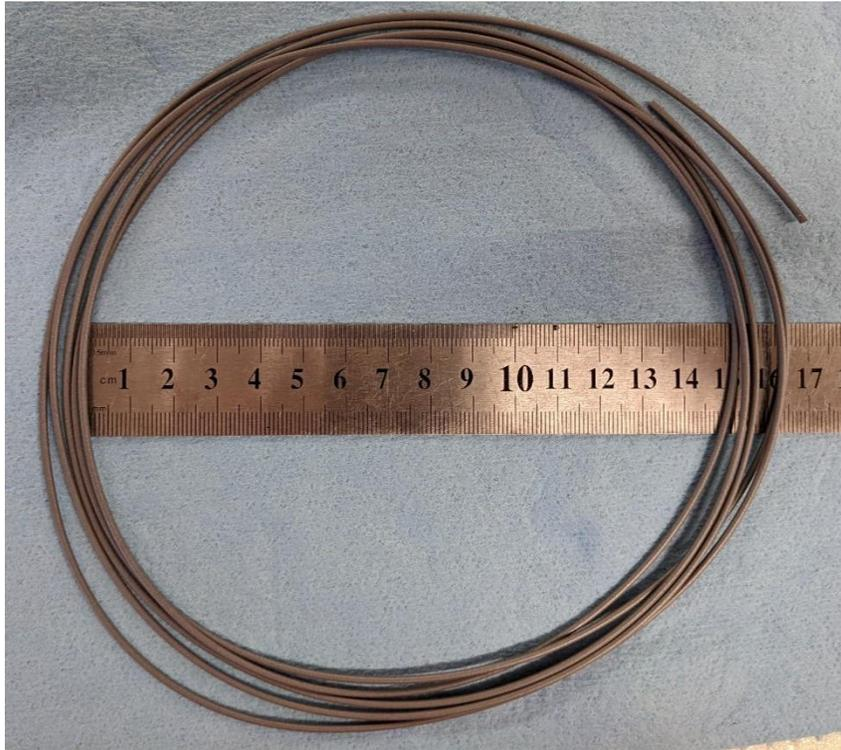
FIGURE 11 - 60 vol% Al-6061 filament with spool diameter of 15 cm.
