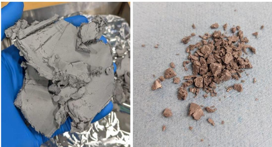
FIGURE 8 - Feedstock batches before and after granulation.
