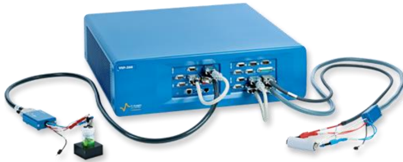
FIGURE 13 – VP300, Potensiostat Device
