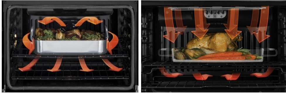
Figure 5-5 The air flow in the oven is controlled by a by the convection fan. Clockwise rotation leads to horizontal air flow configuration(left) and counterclockwise rotation leads to perpendicular air flow configuration (right).
