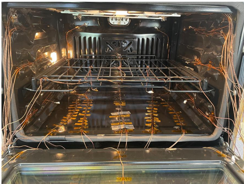
Figure 5-2 Instrumented PTS9000 electric wall oven unit used in study
