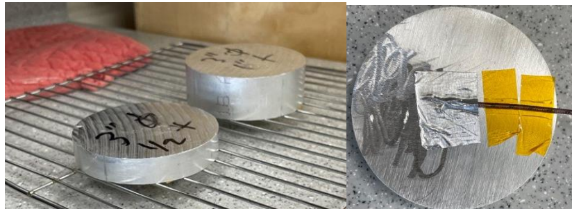
Figure 3-8 Aluminum Discs used for temperature limit testing
