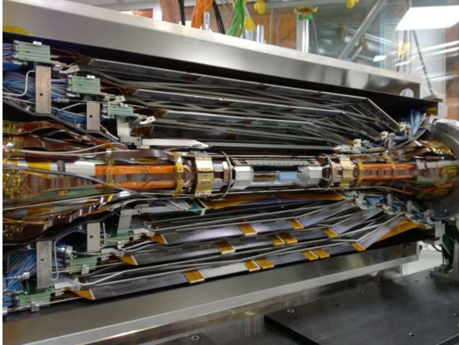
Figure 9. PXD is fitted inside SVD to form the whole vertex detector (VXD) and ready to be installed at the interaction point.
