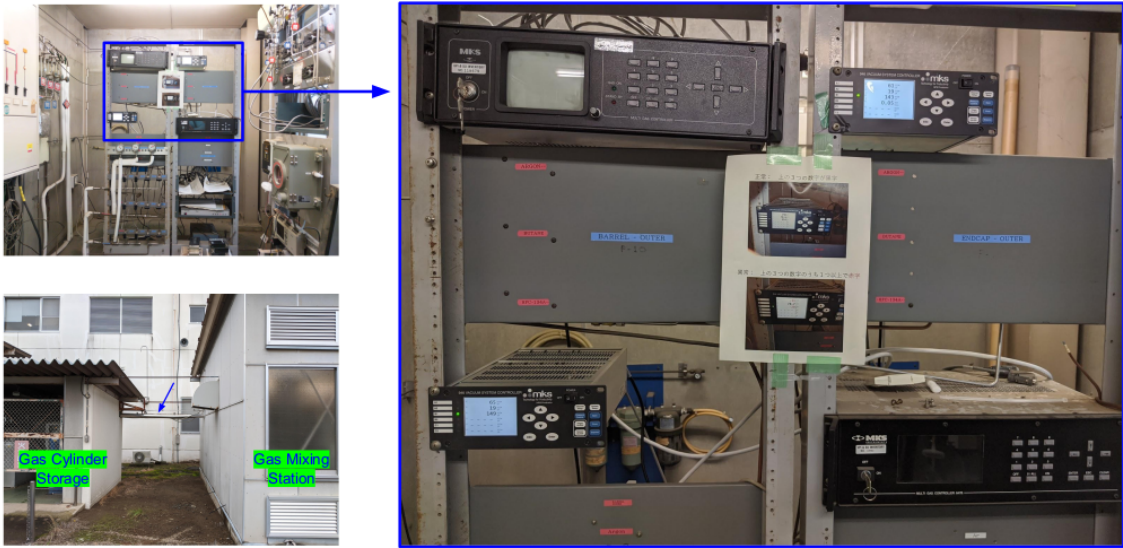
Figure 17. The gas mixing station for the KLM detector, producing a mixture of argon, Freon and butane.
