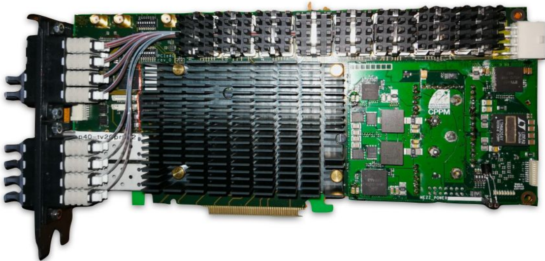
Figure 23. Image of a PCIe40 readout card. There are total 48 slots for belle2link connections, some of them are visible on the left side of the image.
