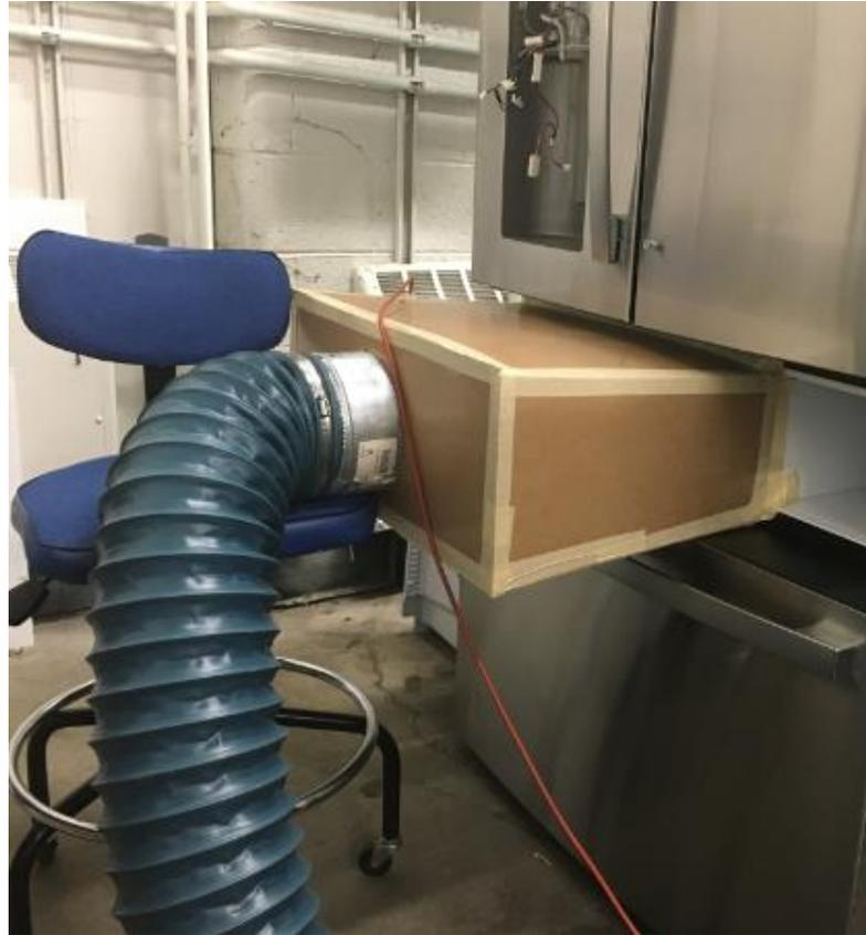
Figure 3-9 Airflow Test setup for convertible drawer flow measurement
