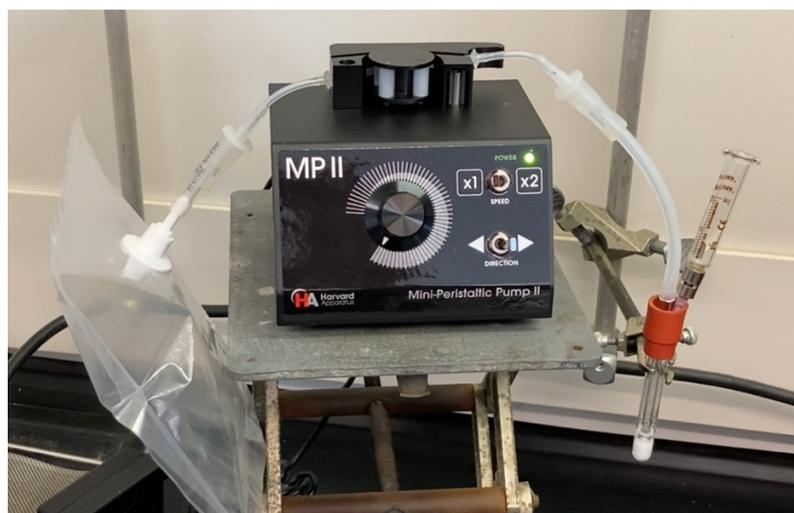
**Figure 2.6A.** Image of laboratory set-up for the reaction of MBA with crotonaldehyde.
