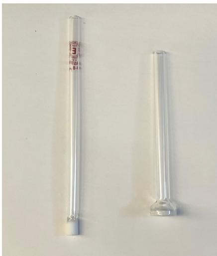
**Figure 2.5.** Image of gas dispersion tubes.
