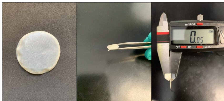
Figure 2.3. Images of the as-prepared polymer-ceramic composite membrane.
