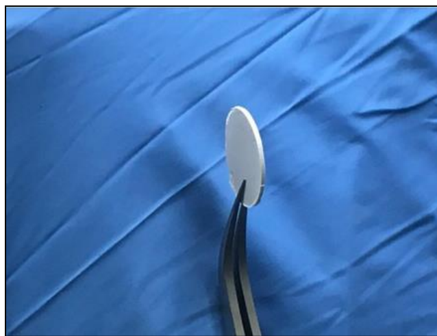
Figure 2.2. A densified pellet made from the cold pressing of argyrodite powders under 480 MPa. Approximately 1/2" diameter and 0.6 mm thick.
