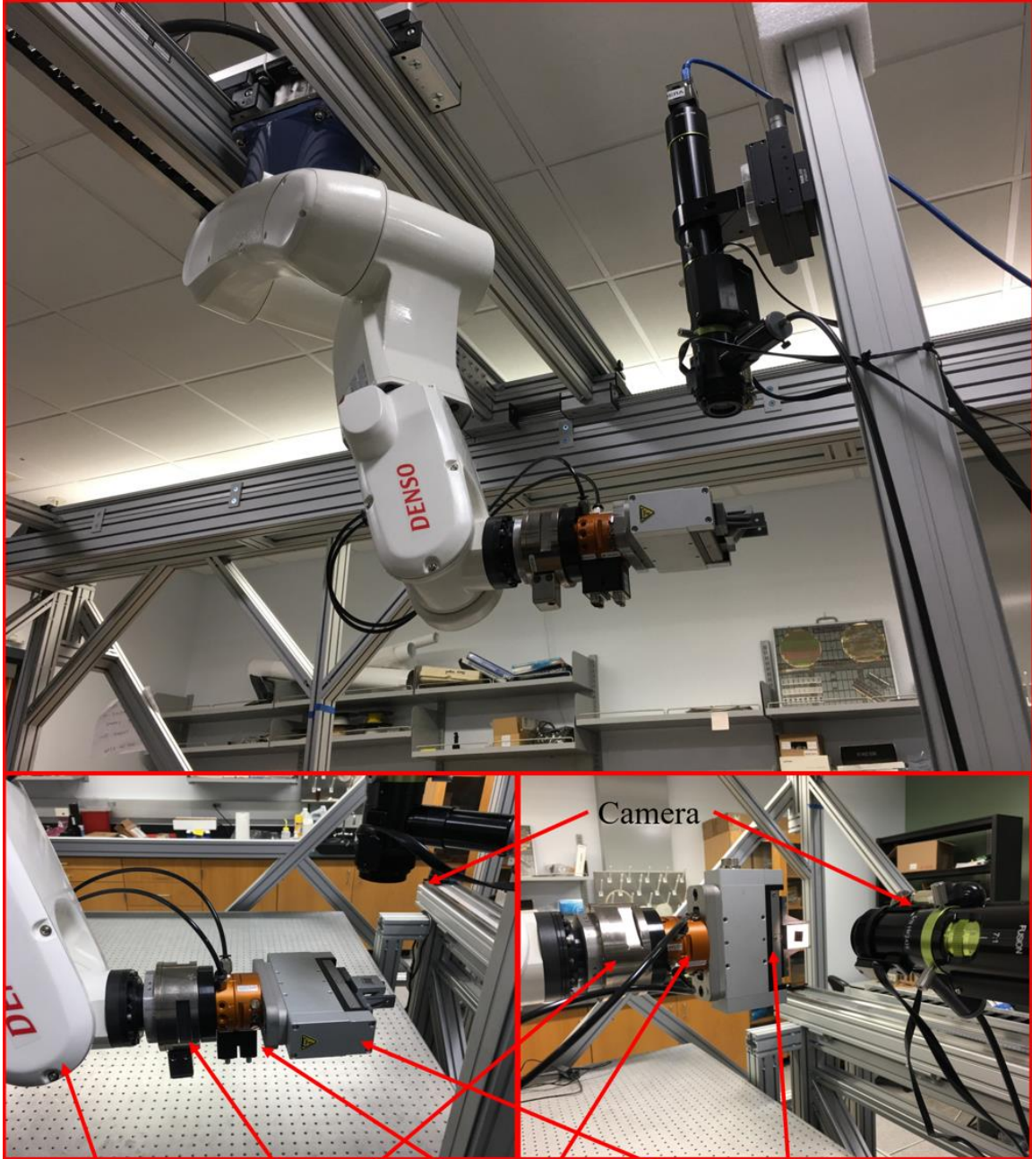
DENSO VS-6577B ATI-Gamma F/T sensor ATI QC-11 tool changer couple HIWIN XEG-32 Electrical gripper
