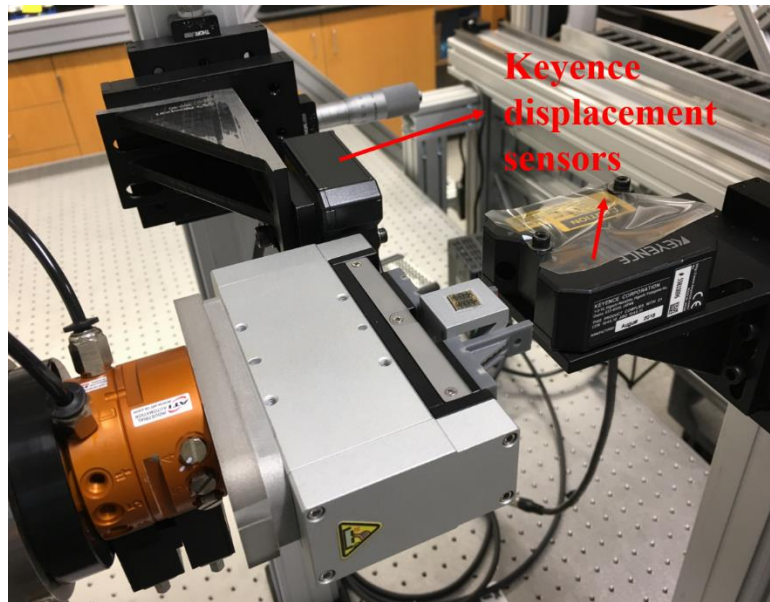
Figure 4. 7 Two laser displacement sensors measure the natural frequency of the robotic arm
