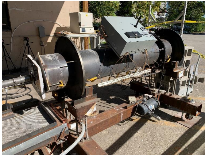
Figure 3: Lab scale rotary kiln setup
