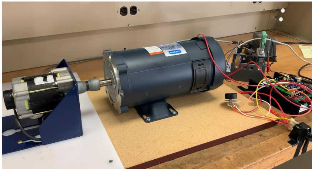
Figure 30 : Motor control bench top testing system
