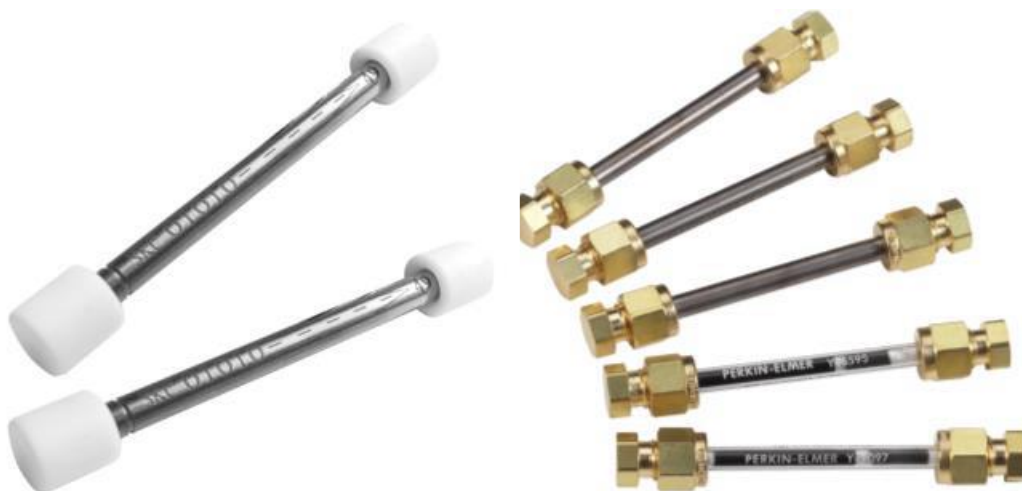
Figure 1.2: (a) Sorbent tube with multiple adsorbents (graphitized carbon black, and Carbosieve S-III) from SKC; (b) stainless steel tube packed with Tenax from Perkin Elmer (copied from Ref. [28]).
