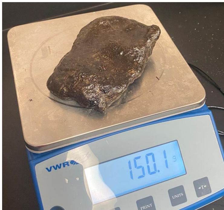
Figure 73 - CdR Recovered from the Foam Fractionation Process
