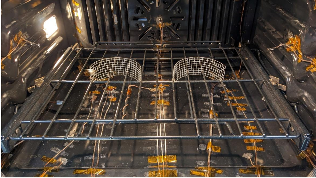
Figure 3-6 Wire mesh modifications made to the oven rack to allow repeatable placement of the cake tins across multiple tests.
