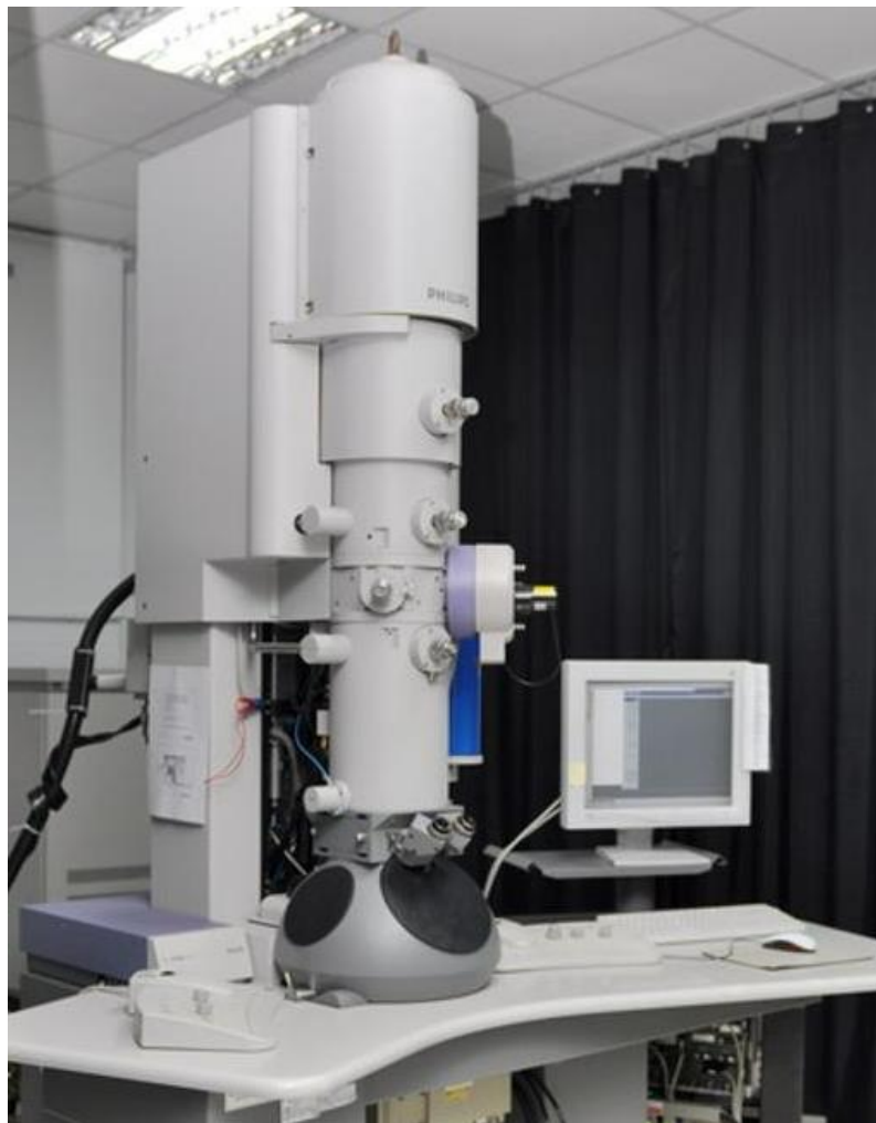
Figure 2.17: FEI Tecnai F20 FEG-TEM/STEM system.
