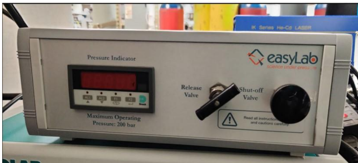
Figure 2.35: GM controller unit
