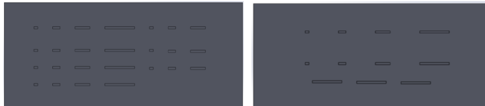
Figure 5.2 Top view of the single tracks of length 0.25,0.5,1 and 2 mm arranged in samples X and Y.
