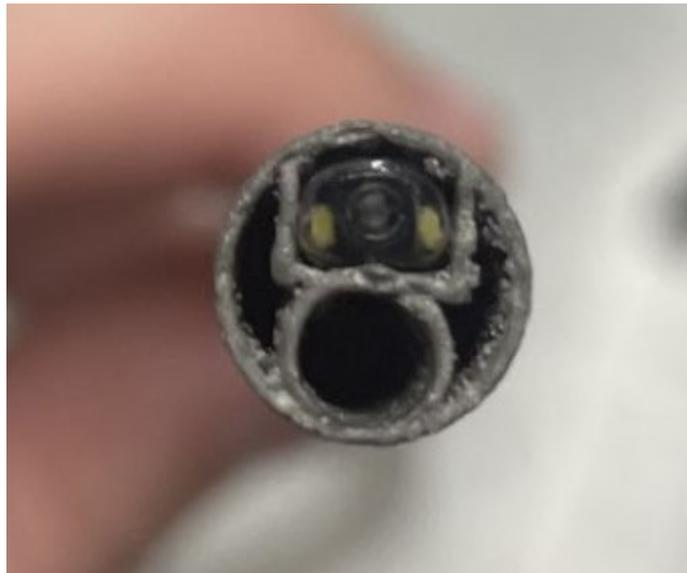
Figure 44: Combined LED light and camera implemented into the shaft of Design VI
