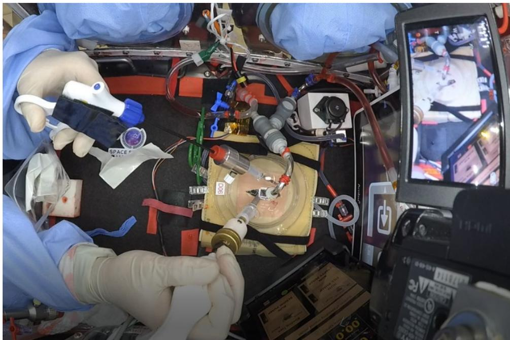
Figure 40: Overhead view of the flight hardware with the MFSD being used inside the surgical containment dome attached to a bleeding wound model
