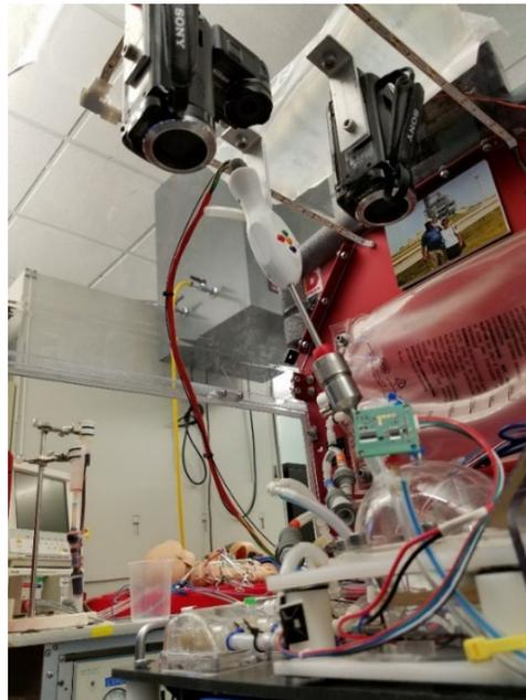
Figure 4: Side view of the University of Louisville suborbital AISS experiment, showing the Design IV MFSD that was implemented for suborbital flight.
