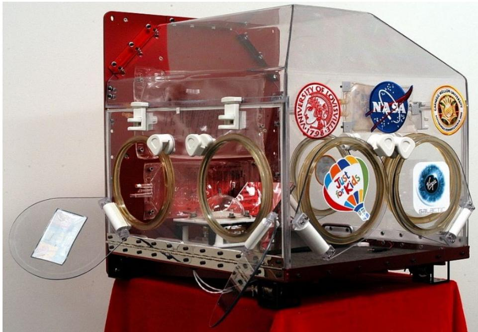
Figure 9: Experiment glovebox with two arm access ports open
