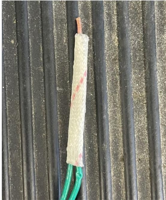
Figure 47: Original cautery element in the fiberglass tubing intended to be implemented into the MFSD shaft
