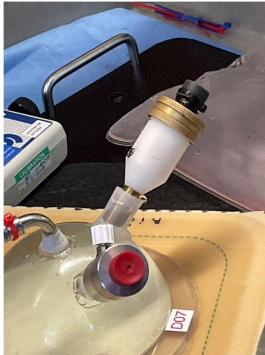
Figure 38: Installed design development model of the final version of the 8mm leak-free trocar.
