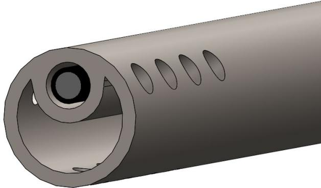
Figure 17: 3D model showing tip of the shaft for the Design IV of the MFSD
