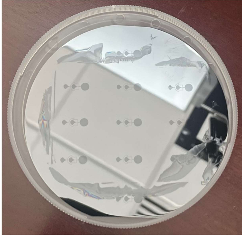
Figure 13: SU-8 mold containing microfluidic devices designed on AutoCAD.
