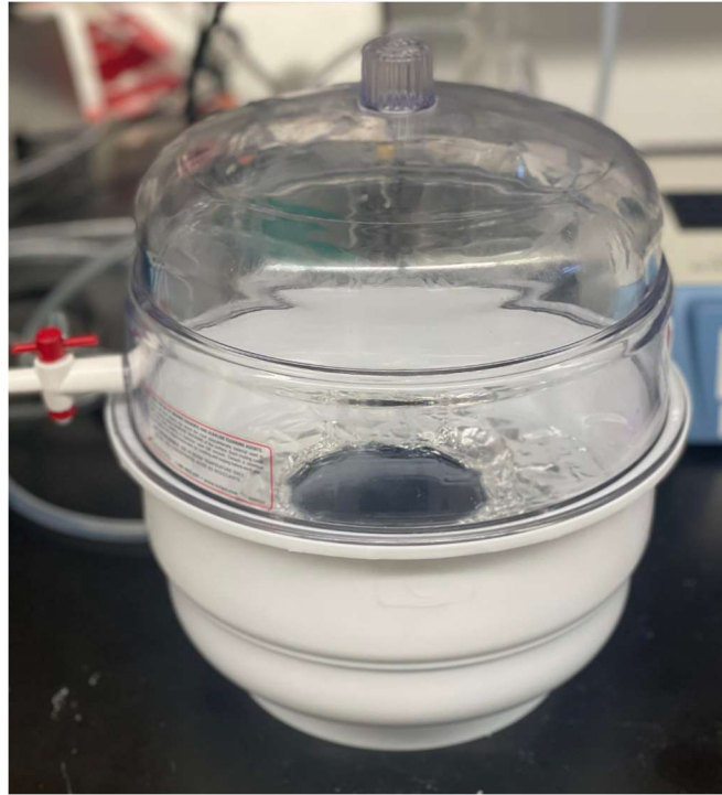
Figure 14: Degassing PDMS after pouring onto clean SU-8 mold.
