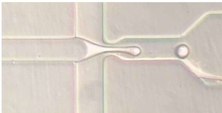
Figures 17-19: Droplet formation within microfluidic device using light microscopy (20X).
