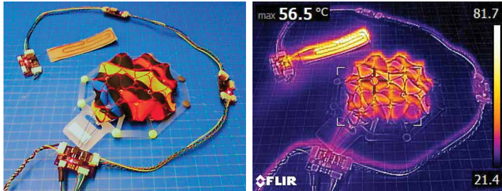
Figure 40. EneGate distributed actuation test.
