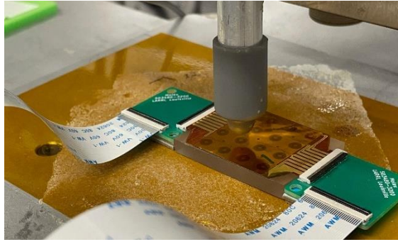
Figure 28 (a) Hardware setup of experimental Testbench (b) closer view of skin sensor testing
