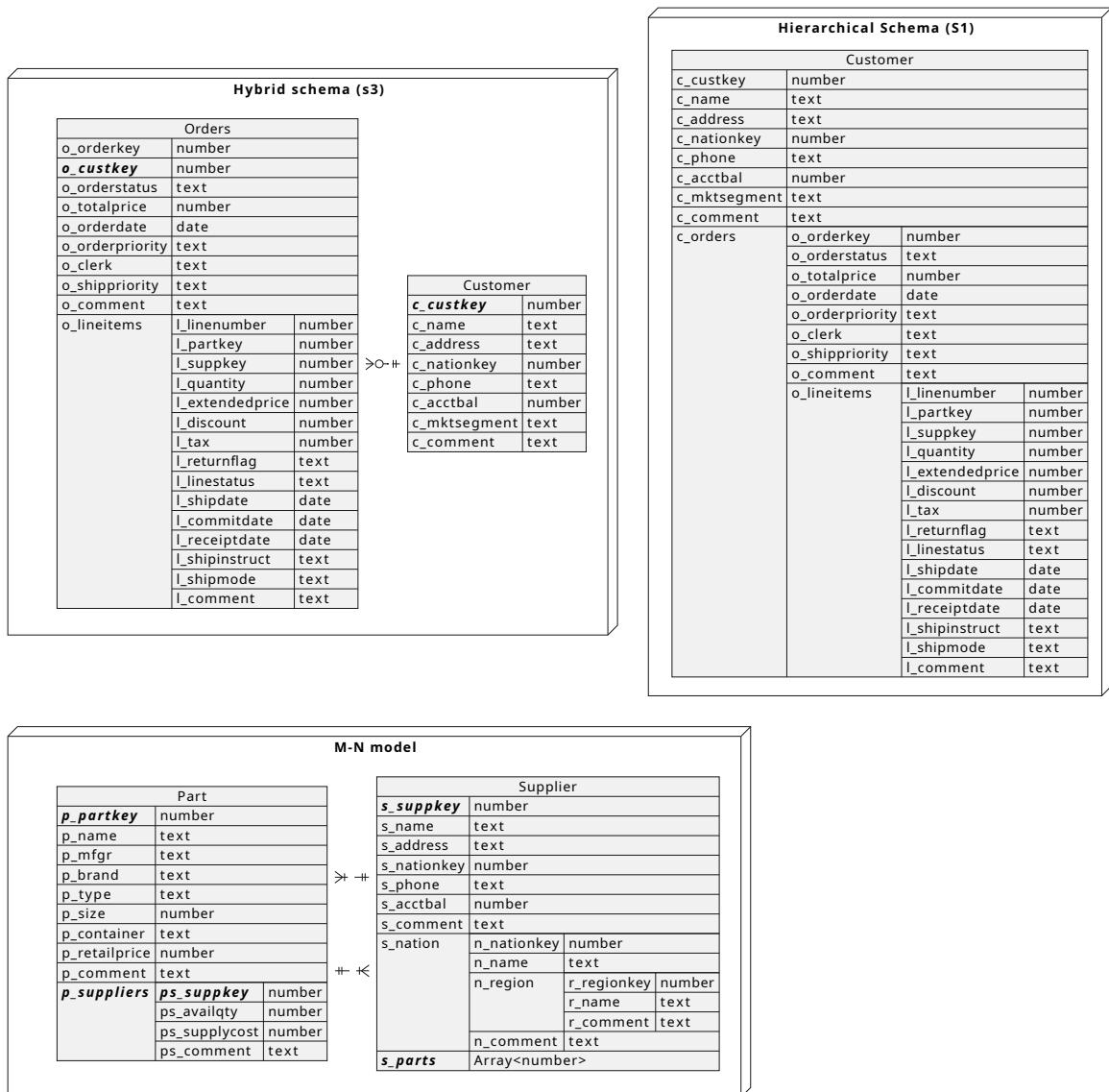
Figure 10. Nested models of the TPC-H schema analogous to the schemas of data used during experimentation. Attributes in bold are used to link the relations
