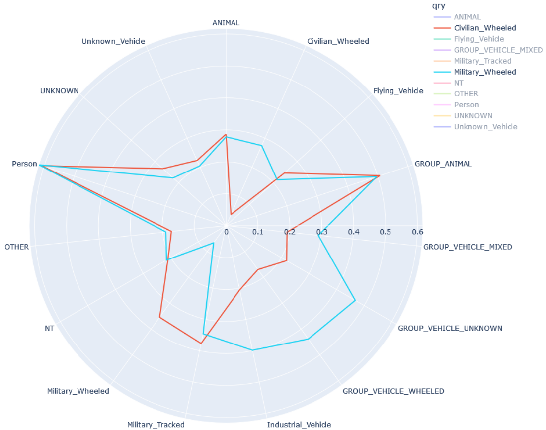
Figure 4.4: Spiderplot isolating Civilian Wheeled Vehicles and Military Wheeled Vehicles. These classes show similar JS behavior for every class other than each other, where we see JS has identified them as distinct classes by their strong self-similarity.
