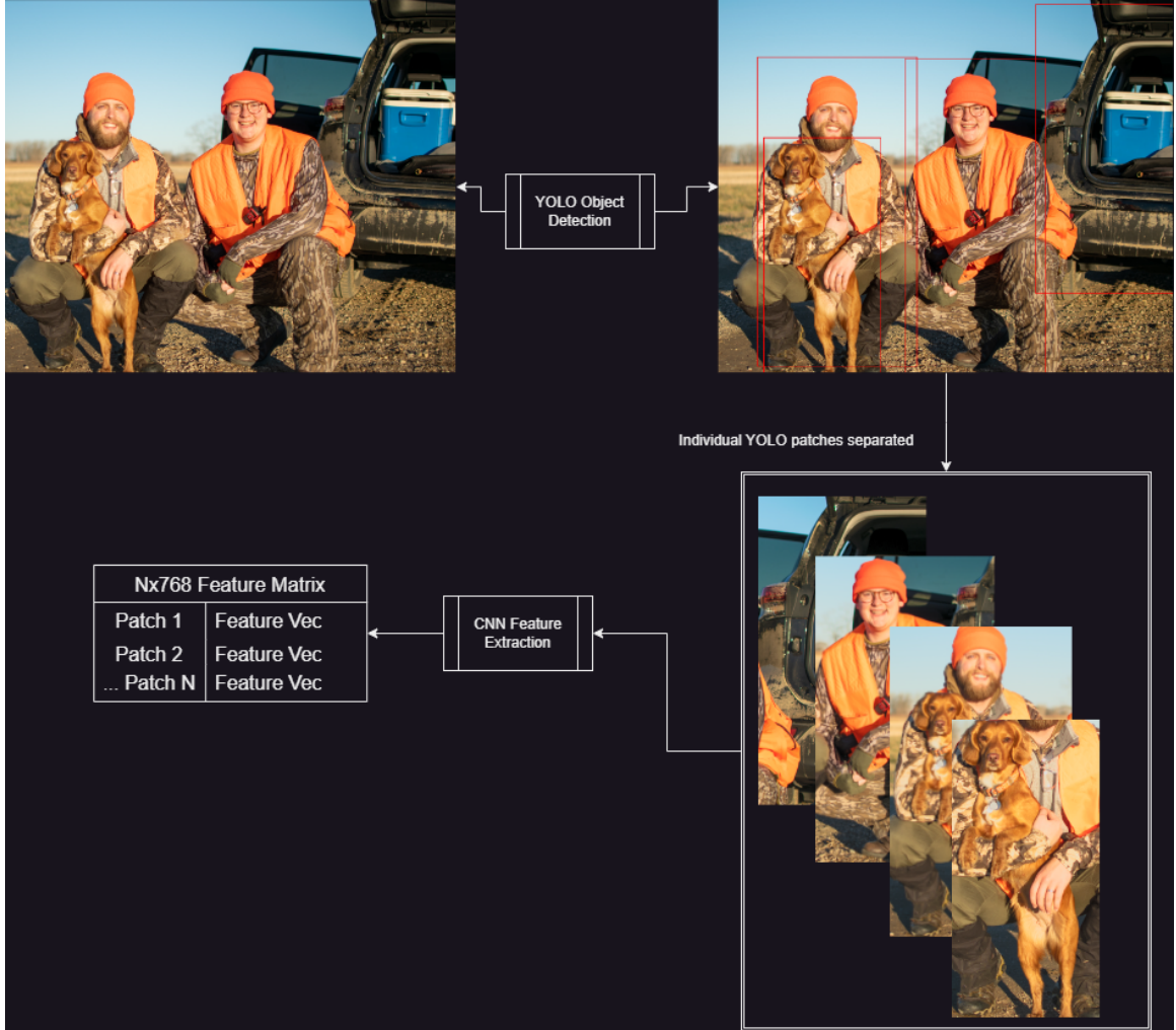
Figure 3.1: Overview of our process to translate a single full image into multiple YOLO-Detected feature patches.
