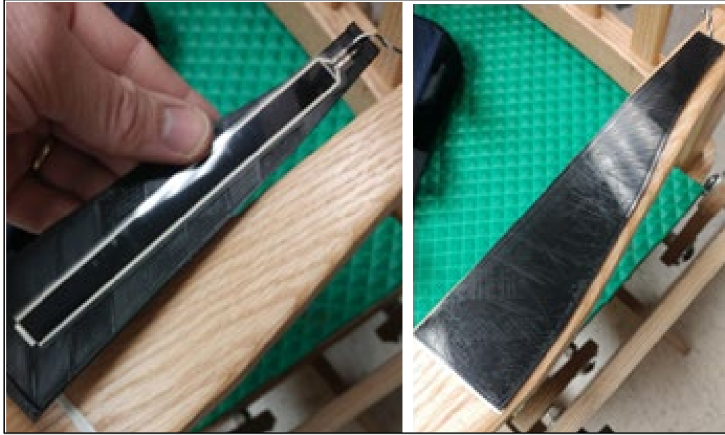
Figure 18: Armrest FSR with 3D Printed actuator
