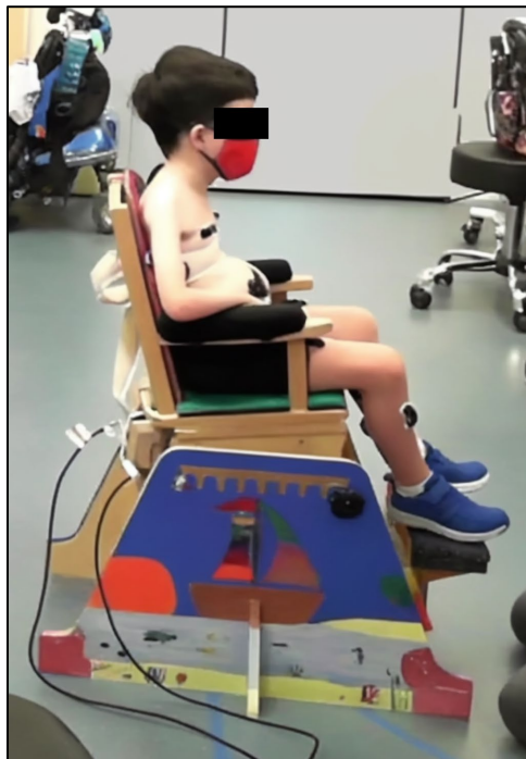
Figure 12: A participant with SCI using the custom rocking chair prototype. Note: strap around chest for support, and footrest raised to support feet.
