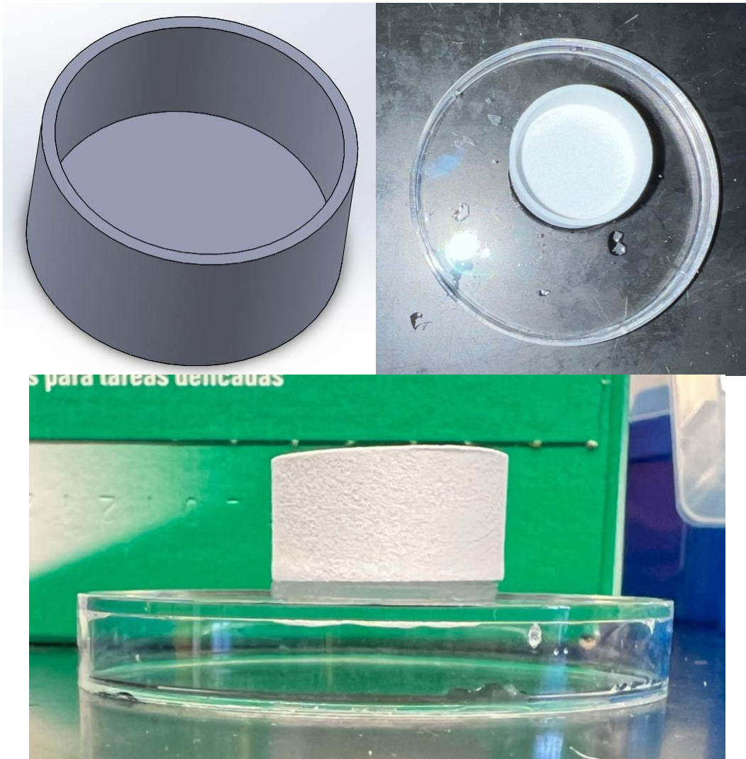
Figure 9. Nylon cup rendering, top view of print, and side view of print atop agarose.
